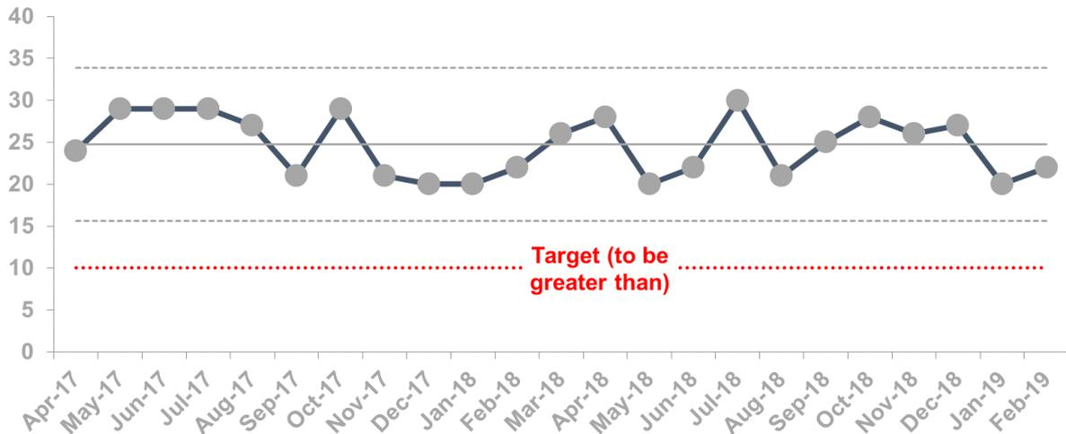
The lower grey dotted line is above the target line. This gives assurance that the target will consistently be achieved, and that the system is effective.
