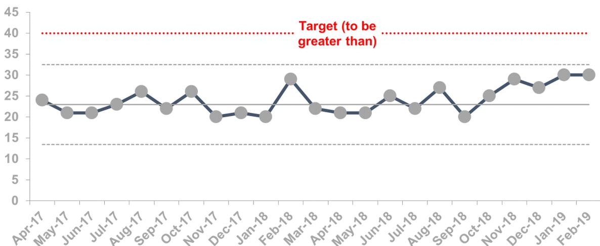
In this example the target is higher than the upper dotted grey line. This means that the target will never be achieved. To achieve the target, we need to change how we do things.
