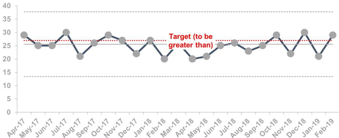
In this example the target line sits between the 2 grey dotted lines. As it is normal for the grey dots to fall anywhere between the 2 dotted grey lines, this means that it is entirely random as to whether or not the target will be achieved. So, this system is unreliable and needs to be redesigned if the target is to be consistently achieved.
